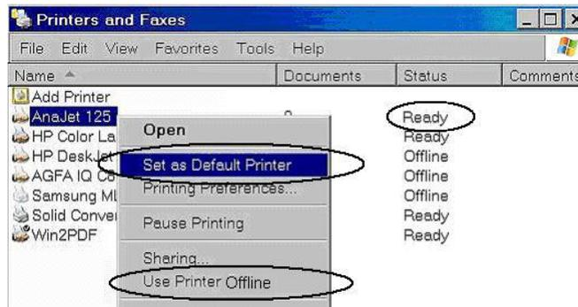
If the MelcoJet does not appear under the Name column, your driver is not installed properly. Notice the Status of MelcoJet. If it is “Offline”, your printer may not be turned on, the USB cable may not be installed correctly, or the printer may have been switched Offline.
