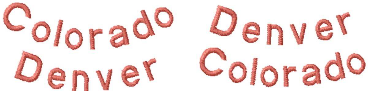
You can also change the arc settings in the DesignShop **View Window**. When **Arc** is selected for the base line type for a lettering object, a radius will be drawn with the lettering (see the following image). You can drag and drop the endpoints of this radius to change the radius length and arc angle.
