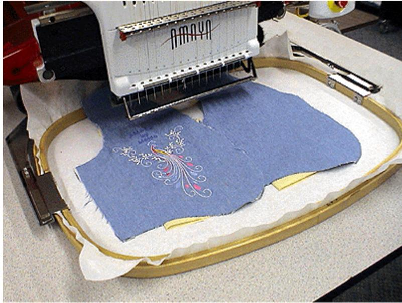
20. When ready to sew on another patch / panel, simply remove the completed patch / panel and place the next one on the double-sided tape.
